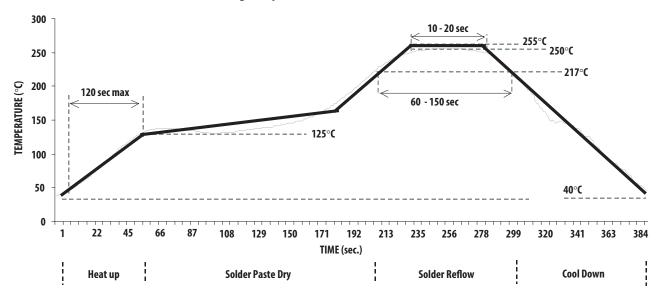
Preheat Temperature 40 °C to 125 °C = 120 sec max Temperature maintain above 217 °C = 60 - 150 sec Peak Temperature =  $255 \pm 5$  °C Time above 250 °C = 10 - 20 sec
