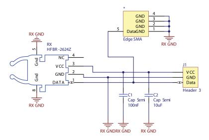
\* Edge SMA connector not assembled.
