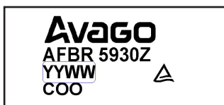
Figure 2b. Component Labeling information
