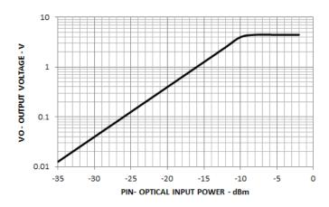
Figure 7 Typical Output Voltage vs. Optical Input Power (Linear Scale
