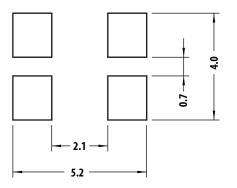
**NOTE:** Recommended stencil thickness is 0.1524 mm (6 mils) minimum and above.
