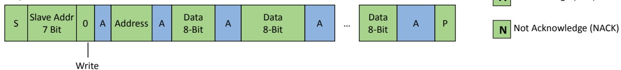
Register Block Write (I 2 C™ Write)
