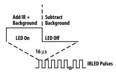
Figure 9. Proximity IR LED Waveform
