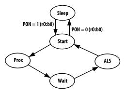
Figure 6. Simplified State Diagram
