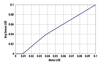
Figure 3c. ALS Sensor LUX vs. Meter LUX using Low Lux Fluorescent Light
