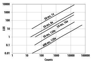
Figure 8. Gain and Integration Time to Lux without IR
