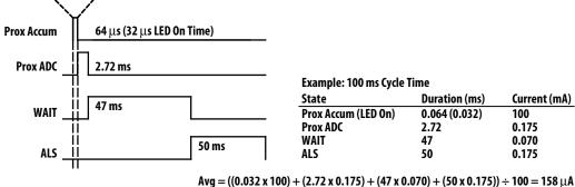
**Figure 14. Power Consumption Calculations**
