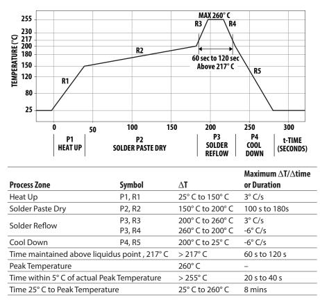
The reflow profile is a straight-line representation of a nominal temperature profile for a convective reflow solder process. The temperature profile is divided into four process zones, each with different  $\Delta T/\Delta$ time temperature change rates or duration. The  $\Delta T/\Delta$ time rates or duration are detailed in the above table. The temperatures are measured at the component to printed circuit board connections.
