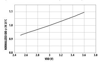
Figure 4a. Normalized IDD vs. VDD
