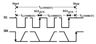
Figure 1. I<sup>2</sup>C Bus Timing Diagram
