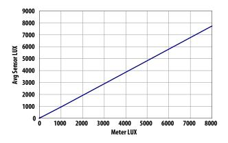
Figure 3a. ALS Sensor LUX vs. Meter LUX using Fluorescent Light
