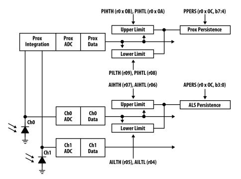
Figure 12. Programmable Interrupt
