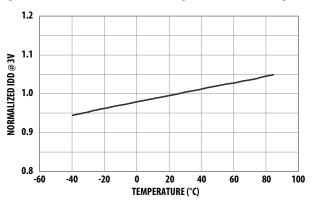
Figure 4b. Normalized IDD vs. Temperature
