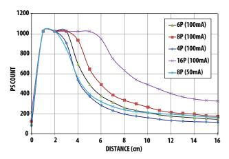
Figure 11a. PS Output vs. Distance, at Various Pulse number (LED drive Current). No glass in front of the module, 18% Kodak Grey Card.
