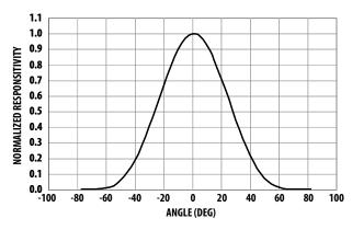
Figure 5. Normalized ALS Response vs. Angular Displacement
