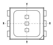
Figure 14: Recommended Soldering Land Pattern
