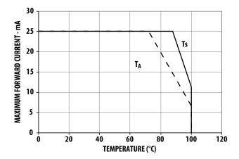
**NOTE:** Maximum forward current graphs based on ambient temperature,  $T_A$  are with reference to thermal resistance  $R_{\theta J-A}$  as follows. For more details, see Thermal Management.
