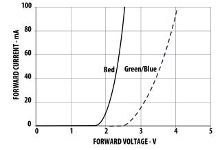
Figure 2: Forward Current vs. Forward Voltage
