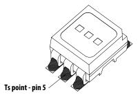
$T_S$  can be measured easily by mounting a thermocouple on the soldering joint as shown in preceding illustration, while  $R_{\theta J\text{-}S}$  is provided in the data sheet. Verify the  $T_S$  of the LED in the final product to ensure that the LEDs are operated within all maximum ratings stated in the data sheet.
