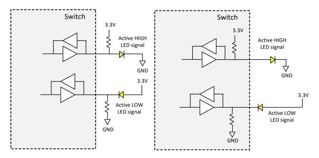
**Note:** When LED signal pins are pulled up or down through an external or an internal termination due to the strap pin configuration, the active states of LED signals are as follows:
