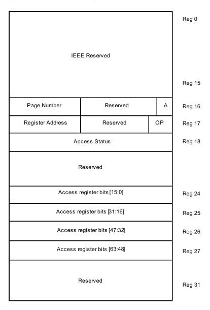
Figure 35: Pseudo-PHY MII Register 16: Register Set Access Control Bit Definition
