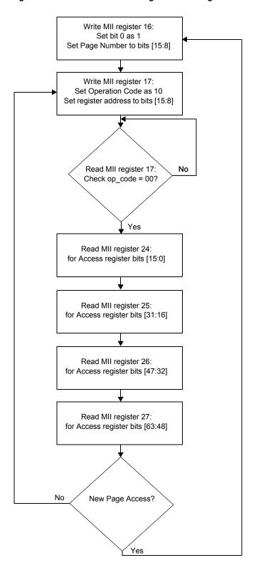
Figure 43: Write Access to the Register Set using the Pseudo-PHY (PHYAD = 11110) MDC/MDIO Path
