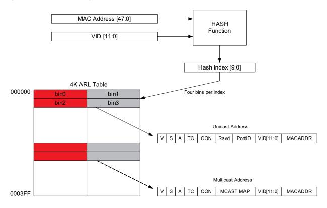
The index to the address table is computed using a hash algorithm based on the MAC address and the VLAN ID (VID) if enabled.
