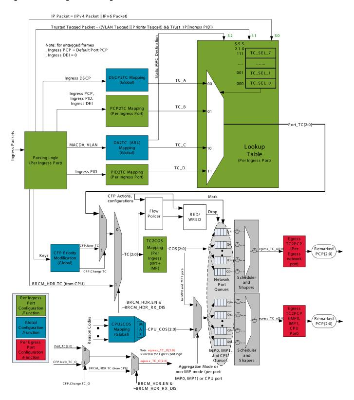
The TC is selected from one of the following sources based on software configuration of an eight-entry lookup table corresponding to the ingress port on which the packet was received.
