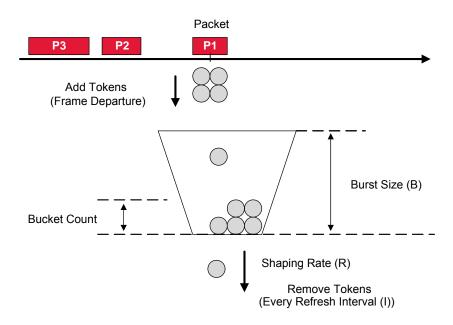
The leaky bucket shaper has the following parameters:
