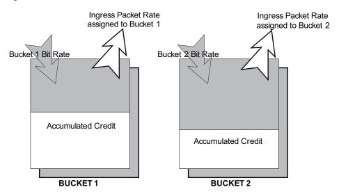
If there is no accumulated credit available, the switch does not accept input packets.
