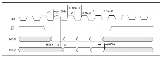
Figure 36: SPI Timings, SS Asserted During SCK Low
