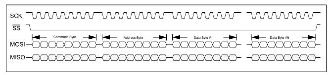
Figure 12: SPI Serial Interface Read Operation
