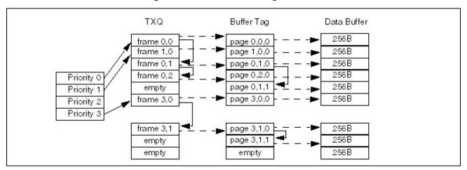
Figure 7: TXQ and Buffer Tag Structure
