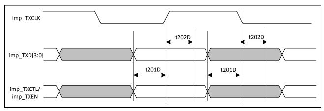
Figure 26: RGMII Output Timing (Delayed Mode)
