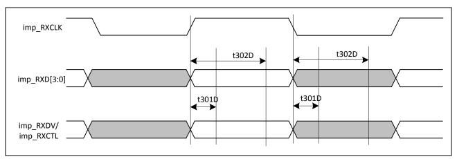
Figure 28: RGMII Input Timing (Delayed Mode)
