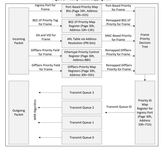
Figure 2: Priority Packet Mapping Flow
