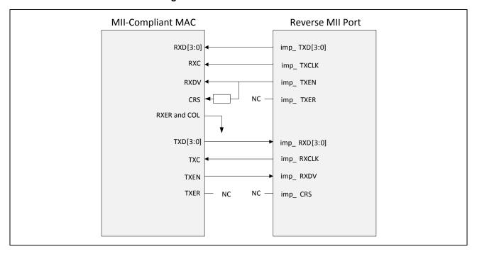
Figure 8: RvMII Port Connections
