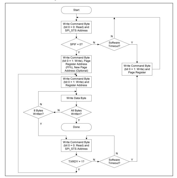
Figure 14: Normal SPI Mode Write Flow Chart
