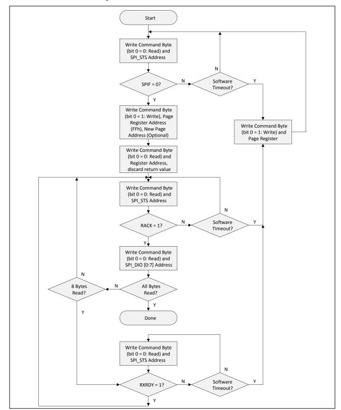
Figure 13: Normal SPI Mode Read Flow Chart
