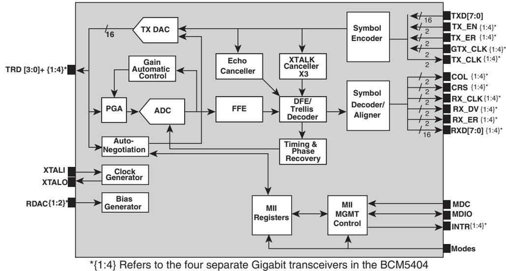
The BCM5421 is a fully integrated 10/100/1000BASE-T Gigabit Ethernet transceiver. The BCM5421 is optimized for low power and small footprint size to enable Network Interface Card (NIC) and uplink applications. By lowering system cost and reducing power dissipation by nearly 50%, the BCM5421 enables a new class of cost-effective Gigabit Ethernet equipment, driving the delivery of Gigabit bandwidth to the desktop.
