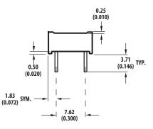
NOTES: 1. DIMENSIONS ARE IN mm (INCHES). 2. UNLESS OTHERWISE SPECIFIED, THE TOLERANCE ON DIMENSIONS IS  $\pm$  0.38 mm (0.015 INCH). 3. LEAD MATERIAL: SOLDER PLATED COPPER ALLOY.
