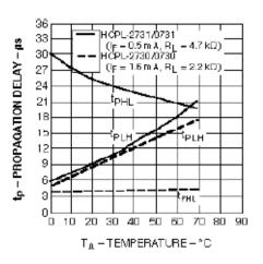
Figure 8: Propagation Delay vs. Input Diode Foward Current
