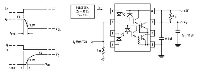
Figure 10: Test Circuilt for Transient Immunity and Typical Waveforms
