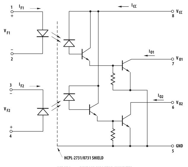
USE OF A 0.1 µF BYPASS CAPACITOR CONNECTED BETWEEN PINS 5 AND 8 IS RECOMMENDED (SEE NOTE 8)
