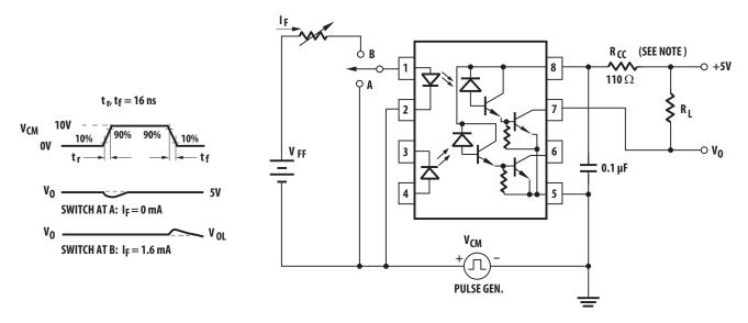
**NOTE:** In applications where dV/dt may exceed 50,000 V/ $\mu$ s (such as static discharge) a series resistor, R<sub>CC</sub>, should be included to protect the detector IC from destructively high surge currents. The recommended value is R<sub>CC</sub> = 110 $\Omega$ .
