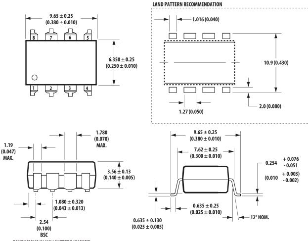
DIMENSIONS IN MILLIMETERS (INCHES). LEAD COPLANARITY = 0.10 mm (0.004 INCHES).
