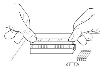
Figure 13: Improper Method to Manually Insert a Display
