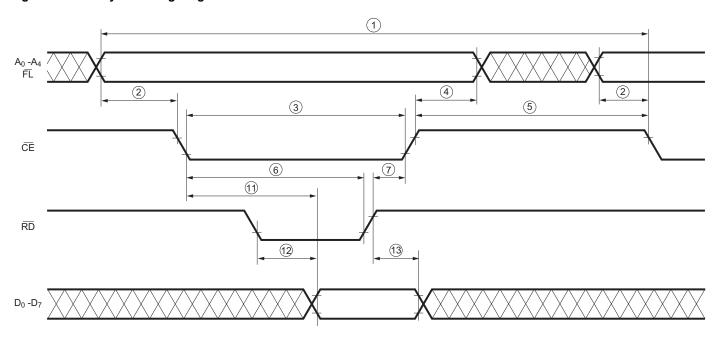
INPUT PULSE LEVELS: 0.6V to 2.4V OUTPUT REFERENCE LEVELS: 0.6V to 2.2V OUTPUT LOADING = 1 TTL LOAD AND 100 pF
