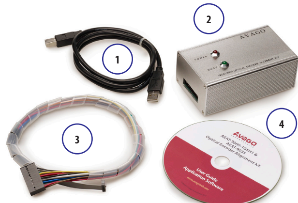
Figure 3. Alignment kit components for HEDS-8969
