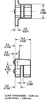
Mounting Option #50 - Standard (Baseplane Mounting) Contact Factory for Detailed Package Dimensions
