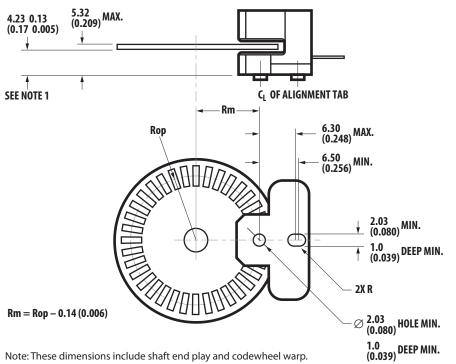
All dimensions for mounting the module/codestrip should be measured with respect to the two mounting posts, shown above.
