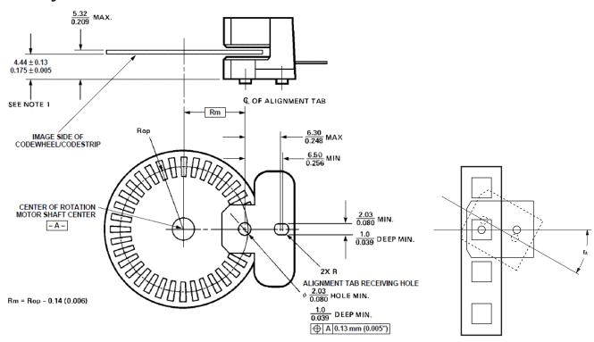
For linear motion, angular misalignment, EA, must be  $\leq \pm 2$  degrees to achieve Encoding Characteristics. All dimensions for mounting the module and codestrip should be measured with respect to the two mounting posts, shown above.
