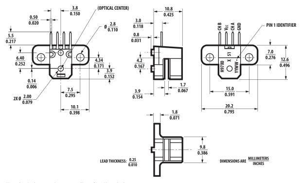
Mounting Option #51 – Screwmount (Baseplane Mounting)
