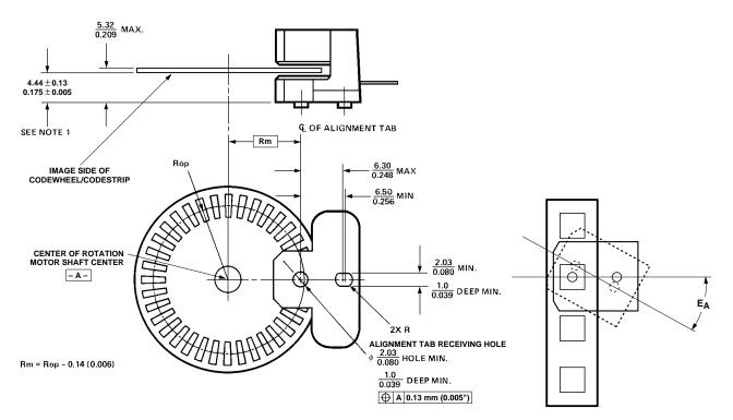
For linear motion, angular misalignment,  $E_A$ , must be  $\leq \pm 2$  degrees to achieve Encoding Characteristics.
