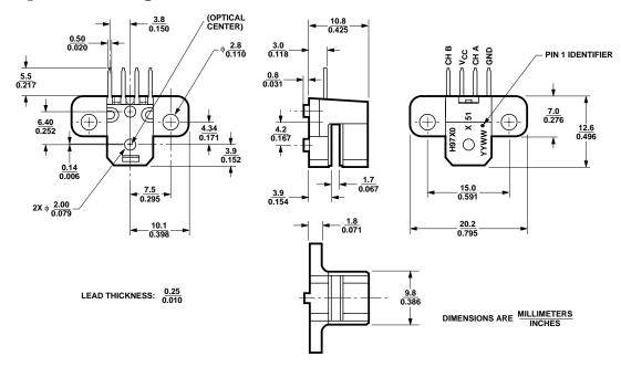
Mounting Option #51 - Screwmount (Baseplane Mounting)
