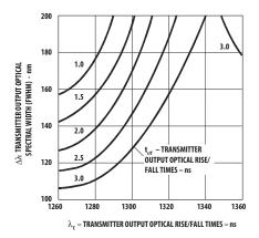
HFBR-5961xxZ TRANSMITTER TEST RESULTS OF  $\lambda_{c}$ ,  $\Delta\lambda$  and  $t_{\it vit}$  are correlated and comply with the allowed spectral width as a function of center wavelength for various rise and fall times.
