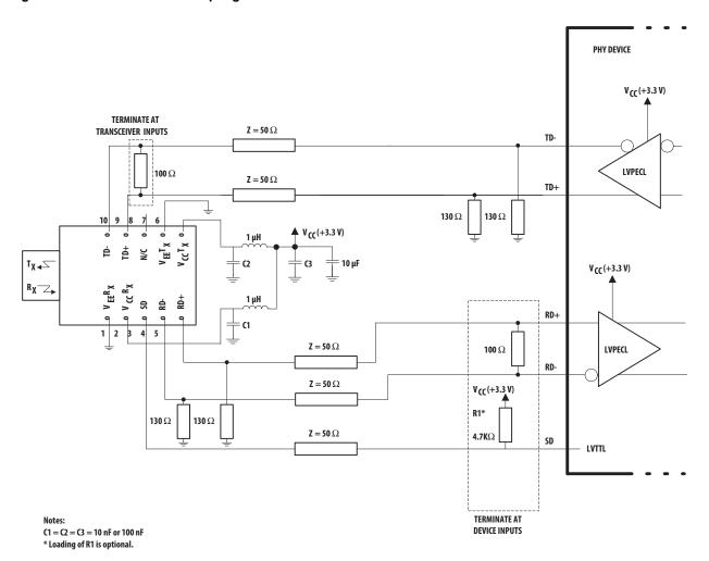
**Figure 4: Alternative Termination Circuits**
