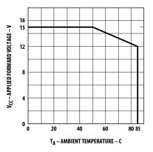
Figure 4. Maximum allowed applied forward voltage vs. ambient temperature  $R\Theta_{JA} = 175^{\circ}$ C/W. 12 volt devices.
