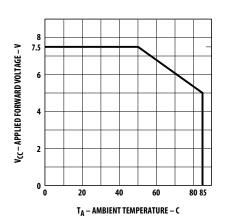
Figure 3. Maximum allowed applied forward voltage vs. ambient temperature  $R\Theta_{JA} = 175^{\circ}$ C/W. 5 volt devices.
