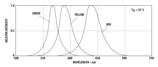
Figure 1. Relative intensity vs. wavelength.
