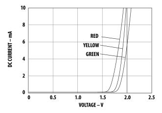
Figure 2. Forward current vs. forward voltage.
