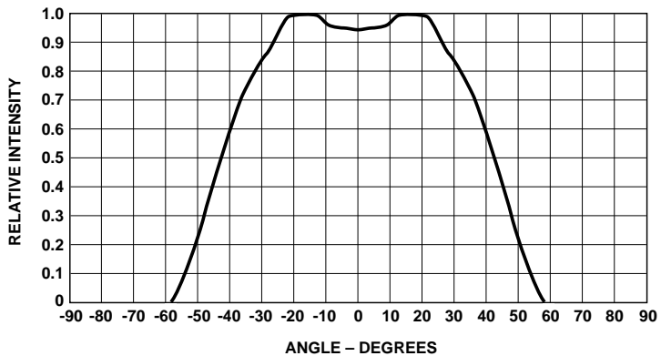
Figure 7. Relative luminous intensity vs. angular displacement for HLMP-Pxxx.
