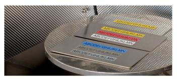
Fade resistant: after laminated labels were placed in a fadeinducing chamber to simulate a year in sunny surroundings, the text was unaffected
