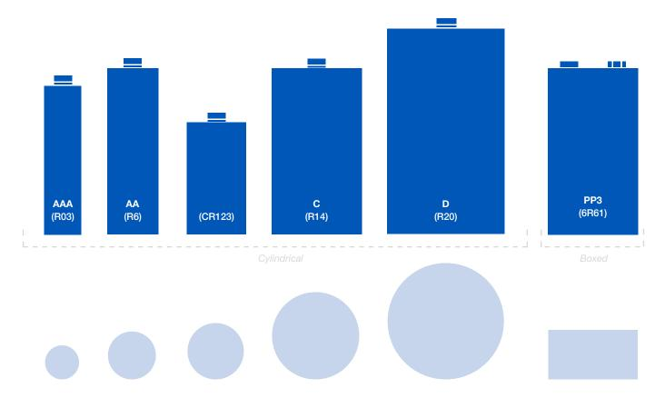
As batteries from different manufacturers may vary slightly in size, Dimensions & Drawings are approximate only. All Bulgin Battery Holders have polarity clearly marked.
