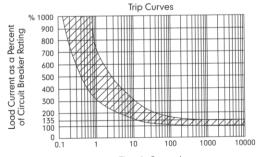
Time in Seconds Trip Curves are Specified at 25°C/77°F
