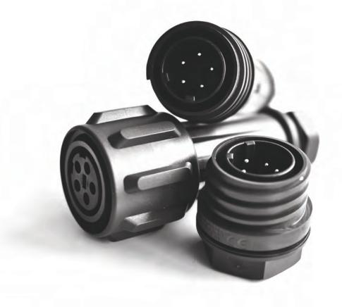
Independently tested for compliance to ATEX standards for use in Zone 2 and Zone 22 environments, the new EXP series is manufactured from a tough,high grade UL94V-0 rated Polyester material and provides environmental sealing to IP68. The ATEX coding is: Ex II 3 GD and the certificated no: Baseefa09ATEX0232X.
