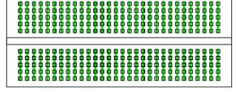
The BB300 breadboard tie-points are connected in 60 vertical columns (the green lines) with 5 connected holes in each. This is the circuit area. When an integrated circuit is plugged into the breadboard, each I.C. pin has a column. There are no horizontal running connections on the BB300.
