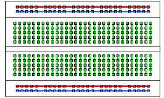
The BB400 and BB400T breadboards have 60 vertical columns in the circuit area (the green lines) plus 4 "rails" or distribution strips for power and ground running horizontally (the red and blue lines).
