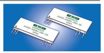
**Type HVD Ultra-Precision Voltage Dividers** are monolithic voltage dividers built with ceramic sandwich construction. These voltage dividers have ultra-precision performance in the range of 1500 volts DC to 5000 volts DC, with a Ratio Tolerance of 0.05% and Ratio TC of 5ppm/°C. These dividers are ideal for high performance voltage division applications in medical equipment, laboratory equipment, analytical instruments, etc.
