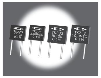
Type TK200 series and TK700 series Low TC Precision Radial Film Resistors utilize Caddock's long proven Tetrinox® resistance system - the first high resistance system to provide a TC that is well within 10 ppm/°C and that is also essentially linear over the entire temperature range from -40°C to +125°C.
