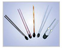
**Pearl-Shaped Precision NTC Thermistor for Temperature Measurement.**The MF52 series is ethoxyline resin coated. The small size is made possible by new materials and manufacturing methods which provide the benefit of close tolerances and fast response. MF52 thermistors are available with 5 lead styles in standard or custom lengths.
