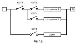
Output 1: must be programmed as an alarm output that is active only for the "Low temperature" alarm. Set "dependence"=c34, which changes from 1 to 9 (or 10 to use normally ON relays). The other parameters for output 1 are not relevant and remain unchanged.
