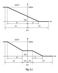
**Mode 6** sees the outputs linked to St1 with "direct" logic ("activation" positive and "differential/logic" negative) when digital input 1 is open. The closing of digital input 1 forces the outputs to depend on St2 and P2, and the logic becomes "reverse", by inverting of sign of the "activation" and "differential/logic" parameters (reading the values of the parameters does not depend on the status of the digital input: these only change as regards the algorithm). When c33=1.
