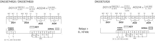
DN33 models with 1DO, 2DO, 1DO+1AO show the complete screen printing, including the outputs that are not available.
