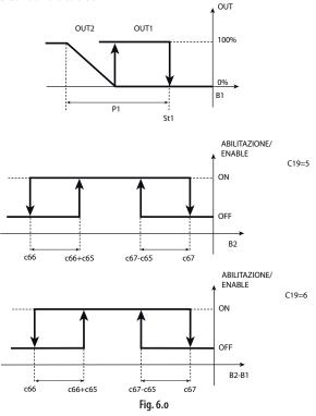
Direct" control with enable logic:
