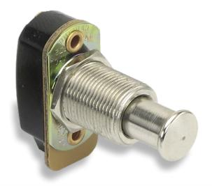
The 16-3P-Series pushbutton switches are single pole and AC rated up to 3 amps. These momentary action switches have a slow-make, slow-break contact mechanism and require only light actuation force (4) oz. - 1 lb.). These switches are typically used in general purpose applications requiring finger actuation.
