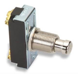
The 170/172-Series pushbutton switches are single pole, high amperage switches suitable for shallow back panel applications. These switches are momentary action and require an actuation force of 2.5 lbs. The 170/172-Series switches are equipped with a slow-make, slow-break contact mechanism and are rated at 15 amps at 125VAC.
