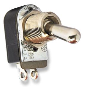
The 110/216-Series is a compactly designed, versatile metal construction toggle switch which is appropriate for a variety of uses. Features include single or double pole options, maintained or momentary construction with termination choices including solder lug end or bottom, wire leads and .250 tab terminals. The quick make/quick break contact mechanism makes the switch suitable for high voltage (125-250 volt) applications.
