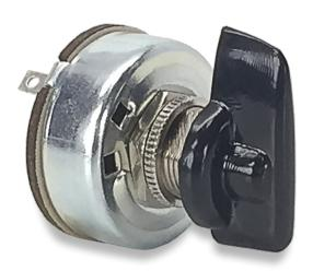
The 700 and 800-Series are single pole multi-position, general purpose rotary switches. These switches feature a nylon actuator in a metal clad construction along with a self-cleaning silver plated contact design. The 700 and 800-Series are typically used in applications requiring multi-position speed controls, such as electric fans.
