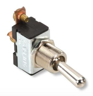
The C-Series single pole compact high current toggle switches are ideal for applications with back panel size constraints. These switches feature self-cleaning contacts and ratings up to 20A 125VAC, 10A 250VAC, 11/2 HP 125-250VAC. With a rugged metal construction, these switches figure prominently in markets with stringent current carrying requirements.
