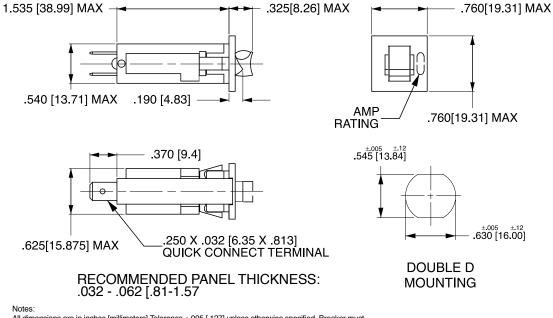
All dimensions are in inches [millimeters]. Tolerance ±.005 [.127] unless otherwise specified. Breaker must hold 100% of rated current and must trip at 150% and above, within the time limits shown in curve. Trip times specified at 25° ambient with no preloading.
