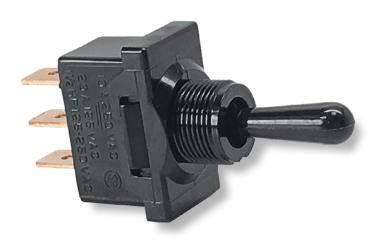
The D-Series single pole compact high current toggle switches are ideal for applications with back panel size constraints. These switches feature self-cleaning contacts and ratings up to 20A 125VAC, 10A 250VAC, 1 1/2 HP 125-250VAC. With an economical double insulated all nylon construction, these switches figure prominently in markets with stringent current carrying requirements.
