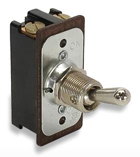
The switch that can handle your heavy duty requirements. Single or double pole with wire lead or screw terminations, and ratings to 20A 125V 10A 250V, the ac/dc DK/EK-Series is the most heavy duty toggle switch in the Carling line. Its sturdy metal construction and stiff actuation force will withstand the abuses of virtually any stringent application. The quick make/quick break contact mechanism is ideal for high voltage DC applications.
