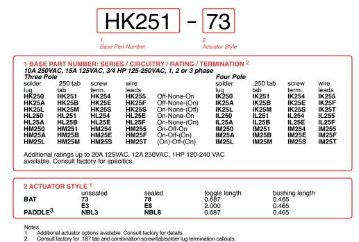
Additional actuator options available. Consult factory for details. Consult factory for .187 tab and combination screw/tab/solder lug termination callouts
