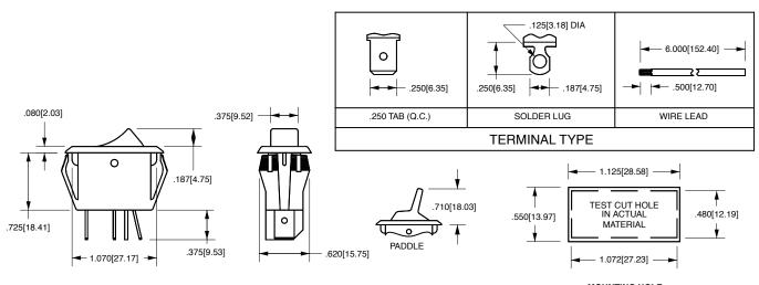
MOUNTING HOLE Panel Thickness: .025 min. - .187 max. Specific cutout dimension range dependent on panel thickness and material. Consult factory
