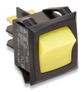
The double pole lighted version of the R-Series incorporates the same sleek lines as the original Curvette, in a double pole envelope. This illuminated version features silver-plated butt-action contacts with ratings to 20A/125, 15A 250VAC and withstand peak inrush currents up to 100 amps. Clear or translucent style rocker actuators and a choice of solder lug, .250 Tab and wire lead terminations enable this switch to adapt to high current applications.
