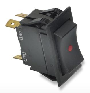
The LS-Series Softspot illuminated rocker switches feature a three-color high brightness light sequence, from a single lamp. These switches are designed with a standard nylon snap-in bracket and "Drip-Dry" construction that protects the front panel from dust and moisture.
