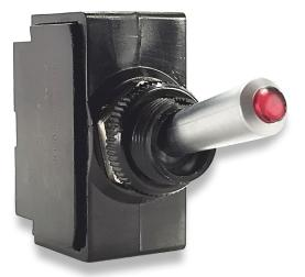
The LT-Series illuminated toggle switches feature up to a three-color lighting sequence from a single lamp. These lighted toggles contain neoprene bushing seals for dust and moisture protection. A variety of circuits and terminations are available.
