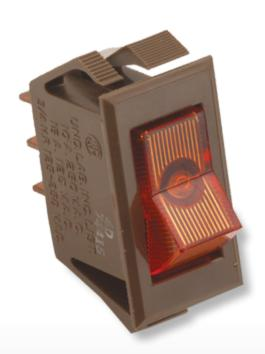
The illuminated predecessor to the Curvette series whose versatility has allowed it to stand the test of time. Traditional styling coupled with self cleaning contacts, integrated wire leads, and various actuator choices has made the LTA-Series appeal to a wide range of markets.
