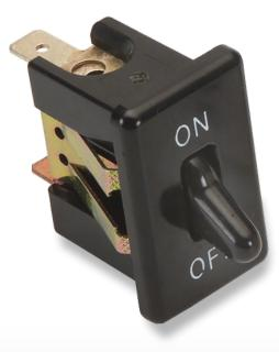
The MAAOA/215-Series toggle switches are single pole, AC rated at 20 amps and 125 VAC. These switches are snap-in mounted, with a phenolic toggle and base, and are suitable for high ambient temperature applications.
