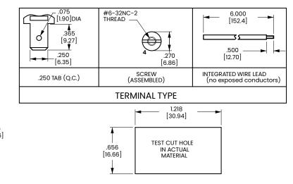
MOUNTING HOLE Panel Thickness: .030[.762] min - .090 [2.28] max. Specific cutout dimension range dependent on panel thickness and material.
