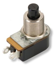
The P26-Series pushbutton switches are single pole, AC rated for 6 amps at 125 VAC and suitable for shallow back panel applications. These switches are momentary action with a medium actuation force (13 oz. typical). The P26-Series switch is equipped with a slow-make, slow-break contact mechanism.
