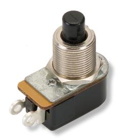
The P26-Series pushbutton switches are single pole, AC rated for 6 amps at 125 VAC and suitable for shallow back panel applications. These switches are momentary action with a medium actuation force (13 oz. typical). The P26-Series switch is equipped with a slow-make, slow-break contact mechanism.
