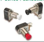
The P27-Series pushbutton switches are single pole, AC rated switches suitable for general purpose applications with a shallow back panel. These switches are momentary action 25,000 cycles with a medium actuation force (26 oz. typical). The P27-Series switch is equipped with a slow-make, slow-break contact mechanism, rated at 6 amps with a nylon concave pushbutton.
